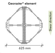
\*) Georaster<sup>®</sup> elements are generally planted with at least 28 plug plants per m<sup>2</sup>. Therefore, there are at least 2 plants in each field of the element. Additonals perennials for visual highlights as per the plant list "Pitched/Steep Pitched Green Roof" are possible. We recommend using vegetation mats or EcoSedum<sup>®</sup> elements for roofs of approx. 30° and upwards.
