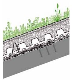
With the Loose-fixed flange construction of the Shear Fix LF 300 and the Eaves Profile TRP 80 even shear barriers within the green roof area can be realised.
