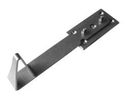
Stable shear retainer, made of solid stainless steel, to be installed on sealed pitched roofs as loose flange / fixed flange construction. Replaces wooden shear barriers in connection with ZinCo eaves profiles.
