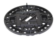
Stackable pedestals made of recycled polypropylene with integrated joint spacers for an easy laying of paving slabs, for levelling facade channels and as support plate in the Elefeet® Support Rail System (= Elefeet® Rail Support Plate incl. screws, Order No. 960053).
