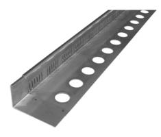
Heavy-duty angle profile made of stainless steel with drainage slots and perforation in the support leg for fixation onto the waterproofing.
