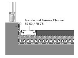
Concrete slabs in gravel bed
