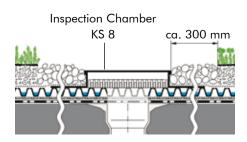
Usually, the drainage of flat roofs is achieved through roof drains. Their quantity as well as their dimensioning is to be determined in accordance with European and German Standard DIN EN 12056-3 and DIN 1986. Inspection chambers make sure the roof drains remain accessible and therefore can be cleaned easily, if necessary.
