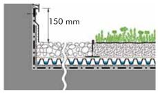
The connection to walls needs to be waterproof. Therefore the protection mat, the waterproofing and the root barrier are taken up at least 150 mm above the finished surface of the green roof build-up and fixed with a protection profile. In front of facades the installation of additional drainage channels is
