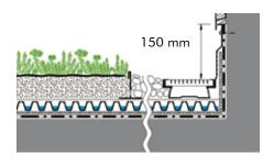
recommanded in order to lead rainwater directly into the drainage layer. If only little water is expected, a simple gravel strip is sufficient.
