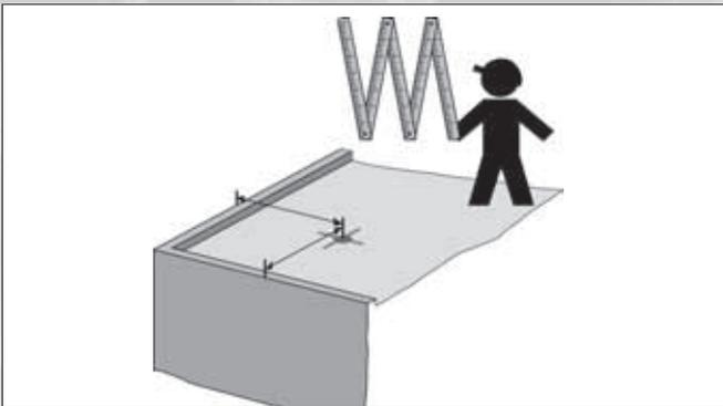
1. Measuring the position of the anchor point
