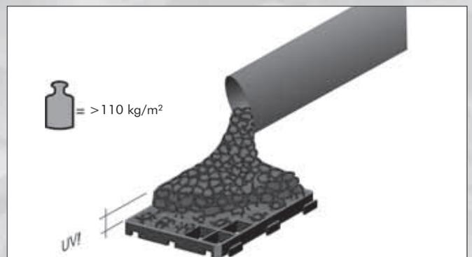
6. Applying the required load (min. 110 kg/m<sup>2</sup>)
