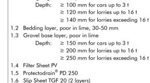
1.7 Roof construction with root resistant waterproofing
