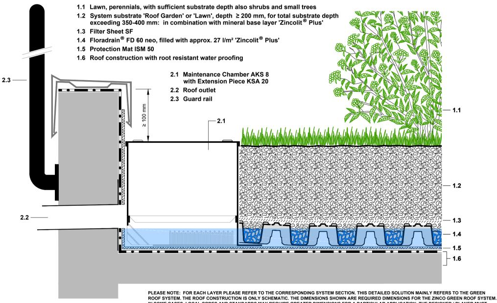
ROOF SYSTEM. THE ROOF CONSTRUCTION IS ONLY SCHEMATIC. THE DIMENSIONS SHOWN ARE REQUIRED DIMENSIONS FOR THE ZINCO GREEN ROOF SYSTEM.
