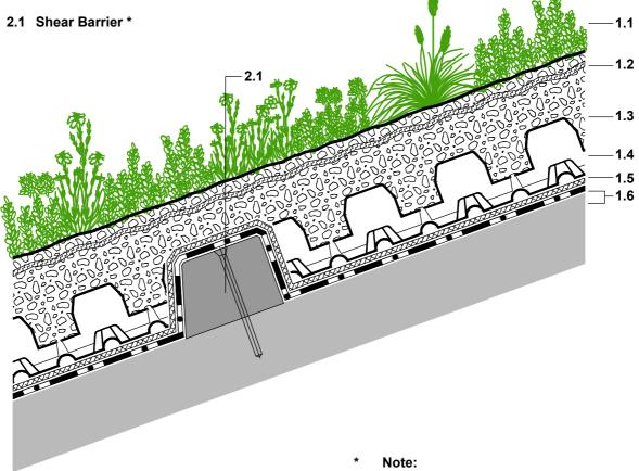
For proper drainage, the shear barrier has to be interrupted every 2 to 2,50 m for 200 to 300 mm
