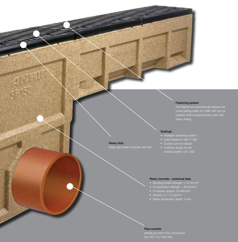
Channel drainage for the load classes D 400 to F 900 According to DIN 19580/EN 1433 "Drainage channels for vehicular and pedestrian areas", these surfaces are assigned to specific load classes depending on the use.
