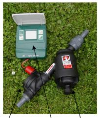
Magnetic valve, computer and filter
